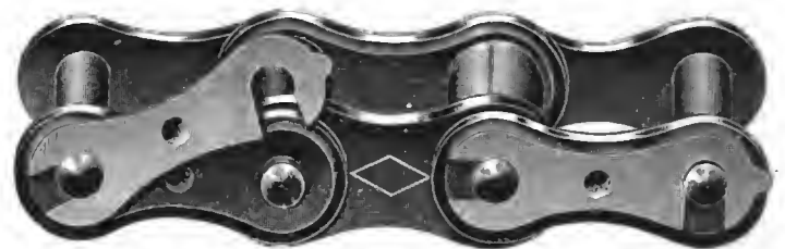
Diamond Detachable Chain Showing Locking Mechanism.
